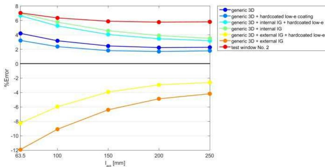
Fig. 2. – %Error in  $U_w$  between 2 and 3D calculation for box type windows with different glazing systems, investigated as a function of leg (the width of the edge-of-glass area)
