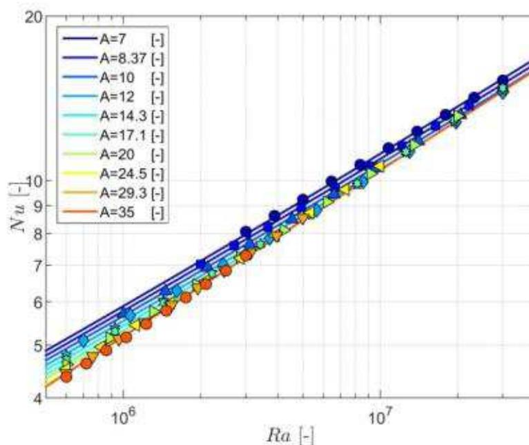
Fig. 1. – the new Nusselt number correlation (derived for the large cavities of double-skin box type windows) compared to parameters study datapoints it is based on
